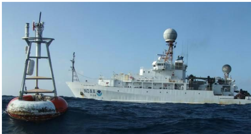
Figure 6: ATLAS mooring buoy and NOAA research vessel, two current means of gathering oceanographic data 7 .
