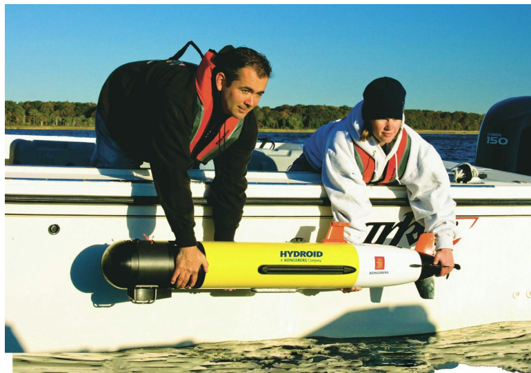
Figure 13: The REMUS 100 autonomous underwater vehicle made by Hydroid, LLC 15 .
