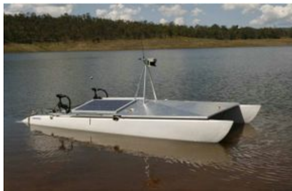
Figure 11: the Lake Wivenhoe ASV, a solar powered catamaran design measuring 16 ft.
