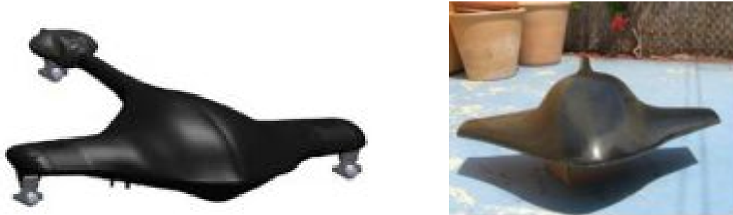
Figure 9: The Stingray AUV: solid model (left) and carbon-fiber hull design (right)
